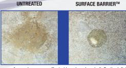
The stone surfaces above were affected by mineral seal oil. On the left (untreated side), the oil has left an immediate stain, while the oil on the right side (treated with SURFACE BARRIER™) has "beaded-up" and can be removed easily without staining the stone.
